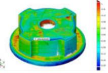
Tested for accuracy We have verified dimensional accuracy within ±0.2 mm or ±0.2% nominal length over the full printer build volume using PPS CF, PET CF, Tough PLA, and PETG.
