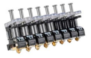
UltiMaker print cores feature a quick-swap design and EEPROM chip. They are recognized by Cura and can be quickly changed without tools to meet the requirements of any print job, increasing your efficiency and decreasing downtime.
