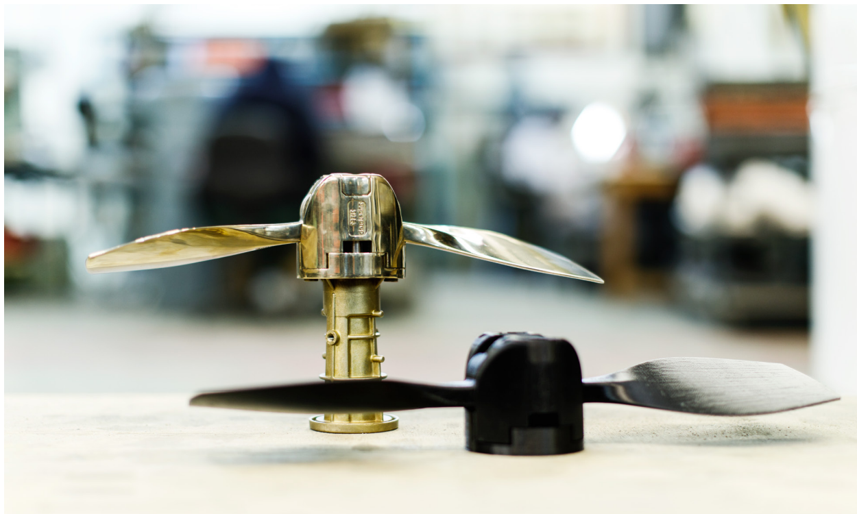
A propeller prototype 3D printed on an Ultimaker printer, next to the final production version
